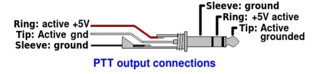
There are separate active grounded and active +5V outputs. The conventional way to control external amplifiers is with a grounded PTT. However the QRP Labs 50W PA kit requires a +5V active (Transmit) PTT control signal. So this PTT output connector is capable of providing both styles of PTT connection.
