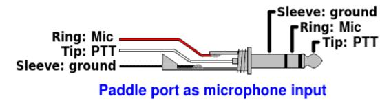
An internal +2.2K pullup to +3.3V is provided to power electret microphones.
