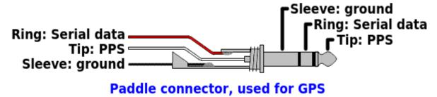
Here the 1pps signal from the GPS must be connected to the 3.5mm jack "tip" connection, and the serial data (9600 baud) to the "ring" connection. In QMX these signals are 3.3V logic level; however they are connected to 5V-tolerant I/O pins on the microcontroller so 5V logic level will also work fine. If you are using a GPS module directly, and it has the common 2.8V output logic, this will also work fine.
