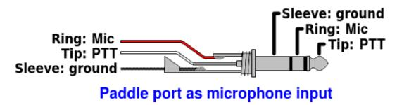
An internal +2.2K pullup to +3.3V is provided to power electret microphones.
