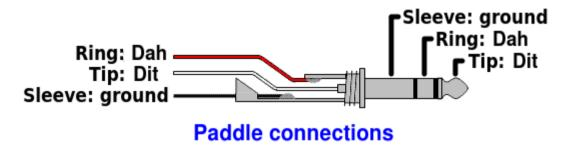
Don't worry if your paddle has a reversed pinout, or if you connect the dit and dah to a 3.5mm jack plug incorrectly: there is a configuration item in the configuration menu (CW Keyer menu) allowing you to swap the dit and dah in the firmware.
