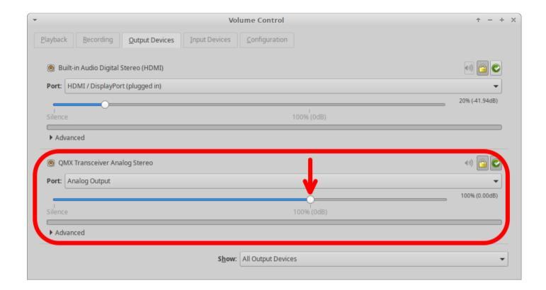
3. The "Master Volume" control of the PC should also be set to 100%. There is such a setting in both Windows and Linux (and most likely Mac too). In Linux, clicking the loudspeaker icon at the bottom right of the screen shows which audio device is being used for the default sound output; selecting QMX will show you the master volume level, and it needs to be set to 100% (not more, not less). There's a similar thing on Windows OS.
