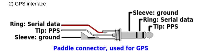
Here the 1pps signal from the GPS must be connected to the 3.5mm jack "tip" connection, and the serial data (9600 baud) to the "ring" connection. In QMX these signals are 3.3V logic level; however they are connected to 5V-tolerant I/O pins on the microcontroller so 5V logic level will also work fine. If you are using a GPS module directly, and it has the common 2.8V output logic, this will also work fine.
