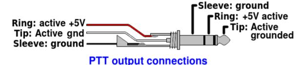
There are separate active grounded and active +5V outputs. The conventional way to control external amplifiers is with a grounded PTT. However the QRP Labs 50W PA kit requires a +5V active (Transmit) PTT control signal. So this PTT output connector is capable of providing both styles of PTT connection.
