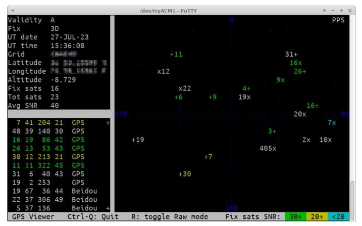
There is a + at the top right of the satellite list panel if you can use the up arrow to scroll up, and a + at the bottom right if you can use the down arrow to scroll down. The example shown here is a QLG2 with its standard active outdoor patch antenna and this is why you see very high SNRs, lots of satellites and both GPS and Beidou. The right-hand panel shows a sky map with all the satellites plotted on it.
