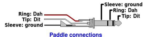
Don't worry if your paddle has a reversed pinout, or if you connect the dit and dah to a 3.5mm jack plug incorrectly: there is a configuration item in the configuration menu (CW Keyer menu) allowing you to swap the dit and dah in the firmware.
