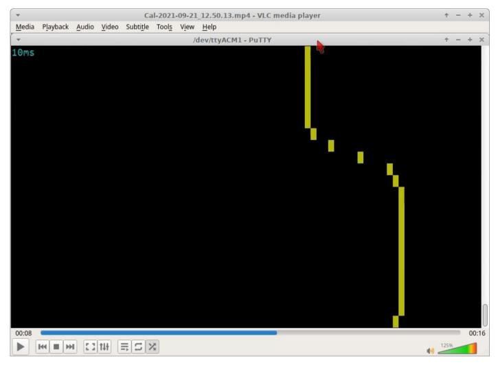
A fun and useful demonstration of the capabilities of QMX and the Input Analysis application, is to investigate the FT8 tone change transition. We know according to the WSJT-X documentation that to avoid splatter onto adjacent frequencies, WSJT-X makes a smooth transition between one tone symbol and the next. It's nice to be able to check this using the Input Analysis screen.
