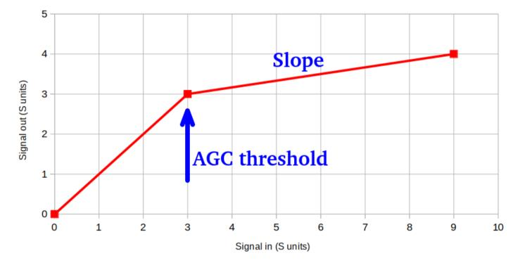
This diagram introduces the first features of the AGC system. An AGC threshold is implemented, specified in S-units. Below this AGC threshold, nothing happens. There is a one-to-one correspondence between the input signal level and output signal level. Practically, I think it makes sense to choose a threshold which is above the band noise level.
