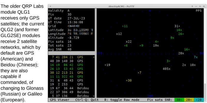
An example display is shown above. There are three panels: top left, some parsed information from the GPS data; bottom left: a list of all the satellites being tracked.
