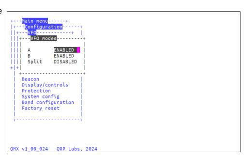
The three settings are available via terminal login (see right) or on the LCD. In the example, VFO's A and B are enabled but Split is not; so pressing the right button will cycle through A and B only, omitting Split.
