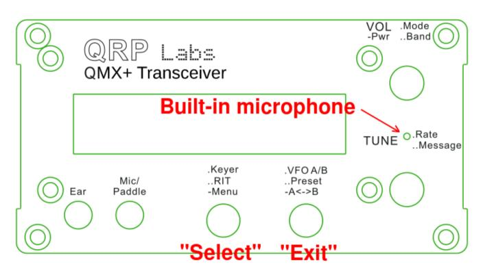
The front panel of the QMX+ has the same controls but they are arranged differently in a Desktop transceiver format, as opposed to QMX where the controls are on the top face of the unit which is more suitable for portable operations.
