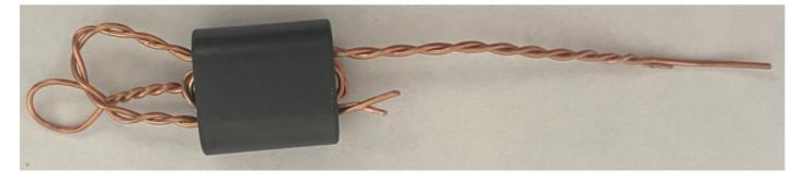
Slide the other twisted pair back through away from the twisted hairpin loop and pull both tight:
