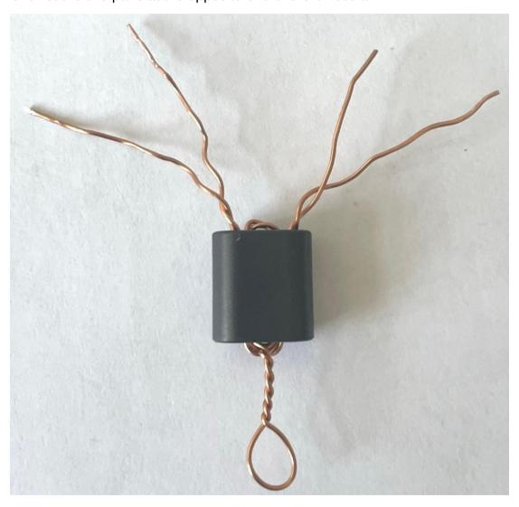
The bottom twisted hairpin loop is the primary, connecting to BS170 transistor drains. Two of the top four wires are the secondary winding, the other two with continuity to the twisted loop are twisted together to form the center tap.
