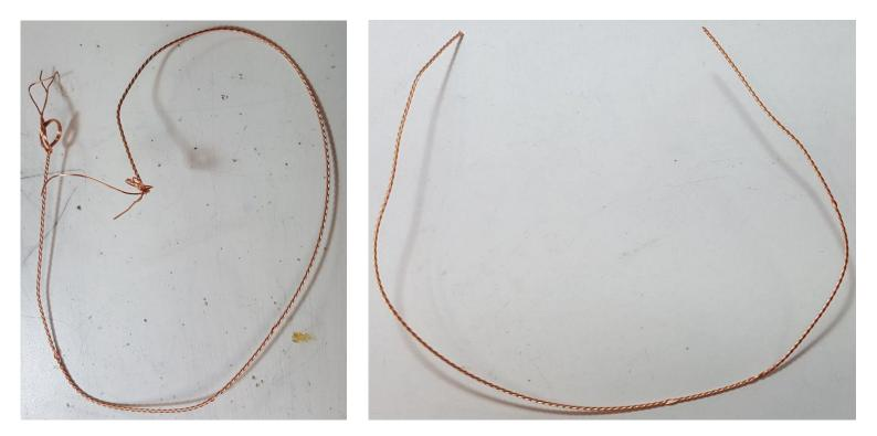
Now cut off the untidy ends, and this is the piece of wire that will be used to wind the FT37-43 toroidal core as a trifilar transformer.
