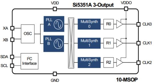
1.46Hz tone spacing for WSPR, on any amateur radio band from 2200m (136kHz) to 2m (145MHz). A 25MHz crystal cannot provide WSPR tone spacing on the 2m band. In summary, the Si5351A chip synthesizes output frequencies in three stages. The block diagram of the chip is shown to the above (from the Si5351A datasheet).
