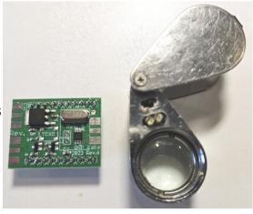
For those using the module in the older Ultimate3 kit (2014 and earlier), make sure there is no pin soldered at pin 12. When using the module in the Ultimate3S kit, you can keep pin 12.
