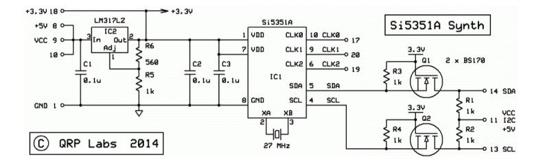
The circuit diagram of the Si5351A synthesizer module kit is shown below.
