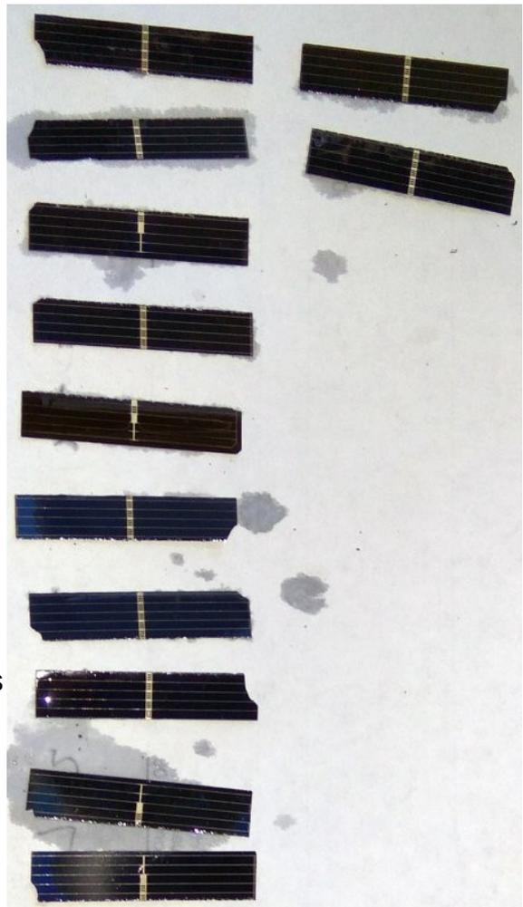
After the glue, the foam base is put on the top of the solar cells and the two pieces of foam with cells in between is inverted. The panels are now loosely glued to the foam base and just a slight movement with a toothpick or similar device can arrange the solar cells perfectly on the foam base. This should be dry in 10-15 minutes.
