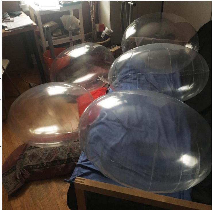
The air pressure is gradually raised using by adjusting the regulator and the humidity should be high to facilitate the balloon stretching. Stretching begins to occur at about .4 psi and the pressure is slowly raised to about 5.5 psi while the physical dimensions of one of
