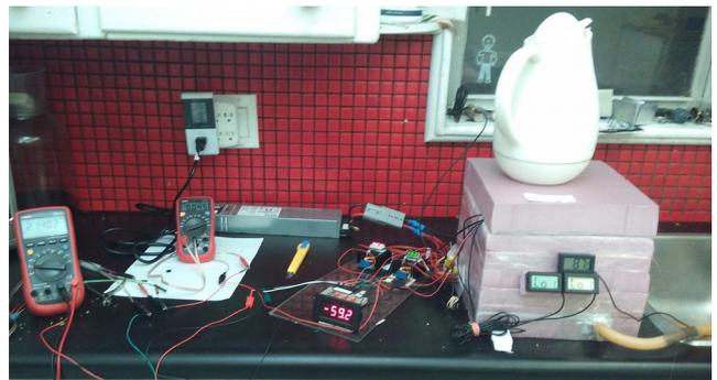
To get the coldest temperature on the top level of the cooler there is a delicate balance of power to each of upper cooling stages. The DC power control to the Peltier stages was
