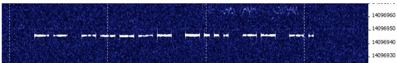
Other variations of the basic principle exist such as DFCW (where the dits and dahs are of the same duration but the dah is shifted up a few Hz compared to the dit) and FSKCW (continuous keying but the real “key-down” is shifted up a few Hz).
