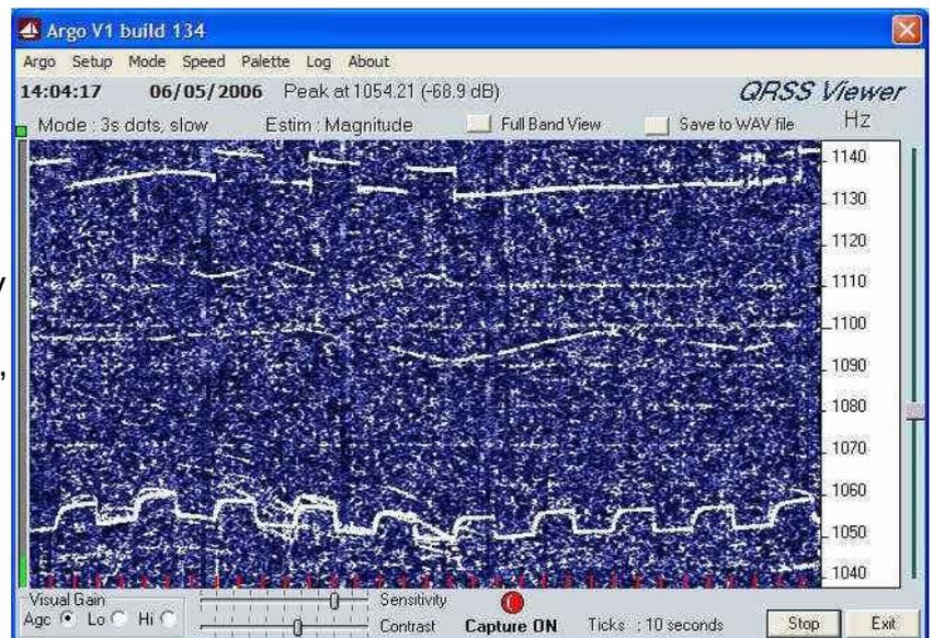
The display shows a small section of audio spectrum, typically only 100-200Hz, displaying the signal intensity in each frequency bucket by the brightness of the pixels.
