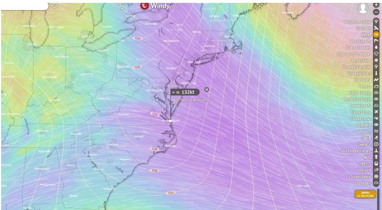
On that same map pressure isobars are shown. The balloon floats higher over high pressure and floats at a lower altitude over low pressure. Wind speed at various altitudes can be shown in a customizable colour scheme. There is a draggable indicator that one can put in the balloon's path to get a good idea of the wind speed. In the image at 11700 meters above sea level. The draggable position flag shows the wind at this moment is 132 knots from the west.
