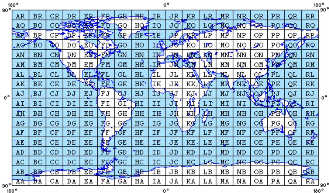
The power level is one of 19 values from 0 to 60dBm, 0, 3, 7, 10, 13, 17, 20dBm etc. The problem is that a Maidenhead grid square measures 1° latitude by 2° longitude. According to ARRL at <http://www.arrl.org/grid-squares>, that is “approximately 70 × 100 miles in the continental US” (110 x 160km). Not only is the location precision very coarse, but we also lack that most crucial of parameters watched by any balloonist: the altitude!
