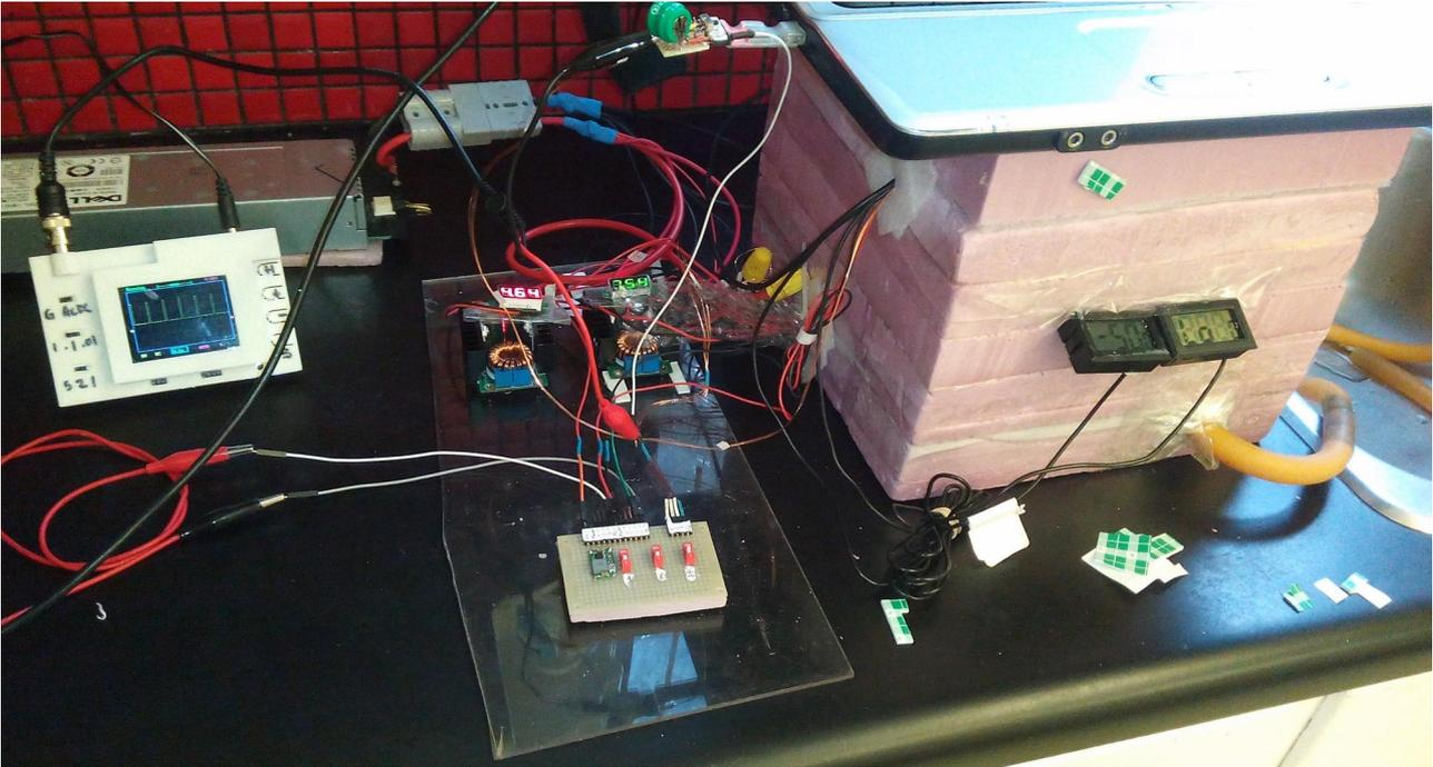
Two cooling stages and the exit water temperature were monitored by simple battery digital thermometers that bottomed out at -50C and then displayed "low". The top or coldest stage was monitored by an analog LM335 chip and a digital calibrated digital sensor.
