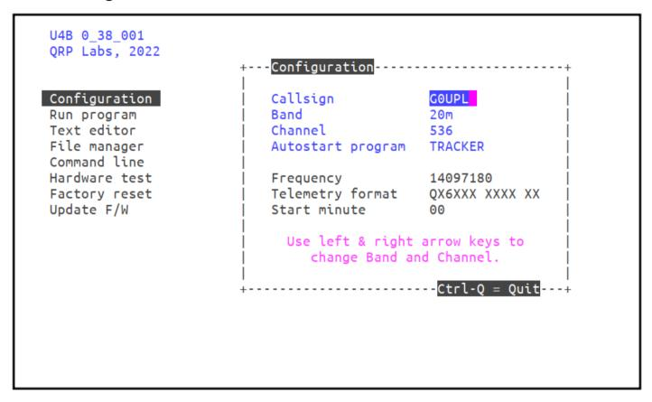
The U4B Configuration screen is where the basic configuration of the U4B tracker and the QRP Labs WSPR tracking system is specified.
