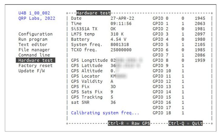
The Hardware test screen provides a comprehensive diagnostic of your hardware.
