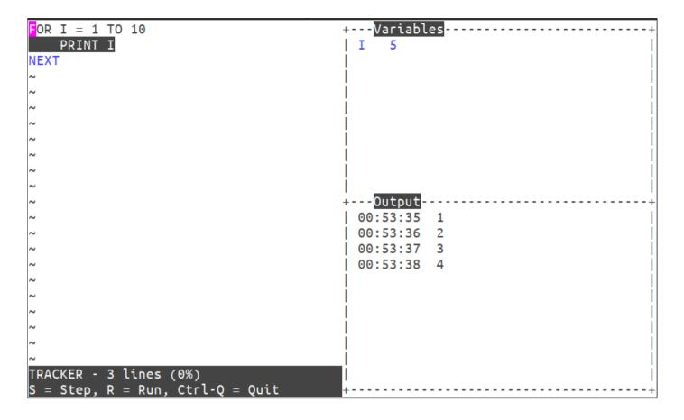
In this example, the S key has been pressed several times. The "Variables" windows hows variable I and its current value, 5. The Output window shows the PRINT statements that have been executed so far.
