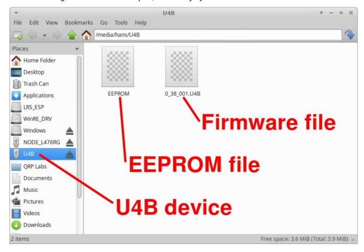
U4B appears as a removable USB Flash device named "U4B", and the folder contains two files. The firmware file shows as a single file which in this example is named 0\_38\_001.U4B. The EEPROM file is always named EEPROM. You can read and write EEPROM files in order to make and restore backup copies of your configuration etc.
