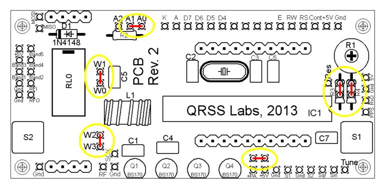
Also pay attention to the jumpers at R3 and R4 on the right-hand side of the diagram. R3 is an optional resistor, to be fitted to enable in-circuit-programming for those wishing to update their own firmware and having the necessary equipment.
