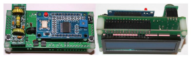
Ensure that the DDS module is inserted the correct way round. The Low Pass Filter kit module should be plugged in with the "Out" legend aligned next to the RF Output connector of the main PCB (see photo).
