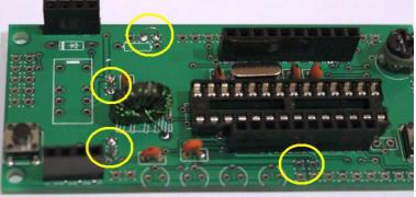
to be removed (for different hardware options configuration), a convenient alternative is to just cut them using wire cutters.
