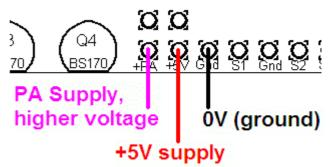
It may be necessary to fix a heat sink to the transistors if the temperature rise is excessive. The transistors are sited near the edge to the board to facilitate this. Experiment is needed in this area, with PA voltages up to perhaps 12V.
