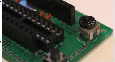
Solder wire jumpers as shown in the diagram below (red wires circled in yellow), depending on your requirements.
