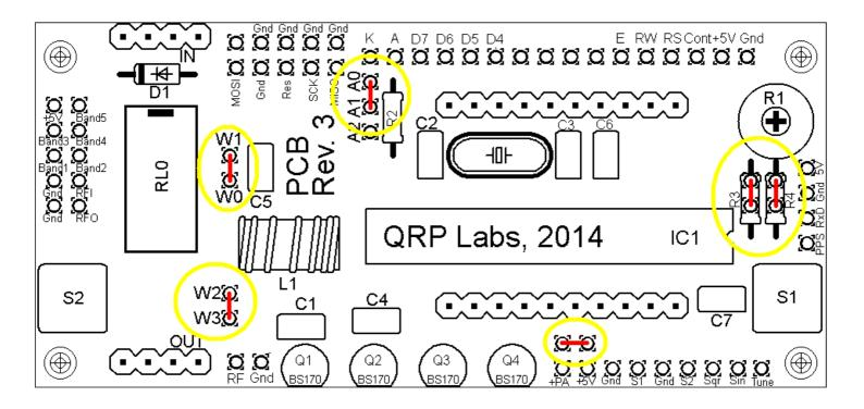
Also pay attention to the jumpers at R3 and R4 on the right-hand side of the diagram. R3 is an optional resistor, to be fitted to enable in-circuit-programming for those wishing to update their own firmware and having the necessary equipment.
