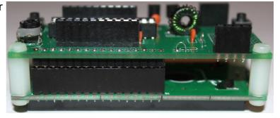
soldered, then you will be able to ensure perfect alignment. Use the eight 6mm M3 screws, and four 12mm nylon hex spacers, to bolt the PCB to the LCD.
