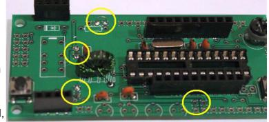
to be removed (for different hardware options configuration), a convenient alternative is to just cut them using wire cutters. PCB Rev 3/4: please follow diagram below, not photo!
