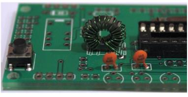
use the DDS and LPF boards plugged into the sockets, then solder the pins, to ensure correct alignment.
