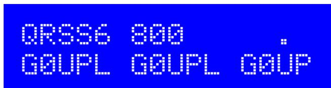
Here the display shows the scrolling message, with a – or a . (for dah and dit), to show which character and symbol is currently being transmitted. The dit speed follows the mode (QRSS), in this example 6 second dits. The frequency is as for FSK/CW (see above) – in this case 800Hz audio output.
