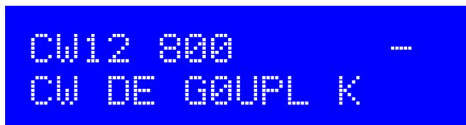
CW mode is just plain, ordinary on/off keyed CW (morse code) at ordinary speeds. The display will show CW followed by the speed – in this example, 12 words-per-minute (wpm), followed by the message which scrolls to the left as it is sent. The character position right before the message shows – or . depending on whether a dah or dit is being sent.
