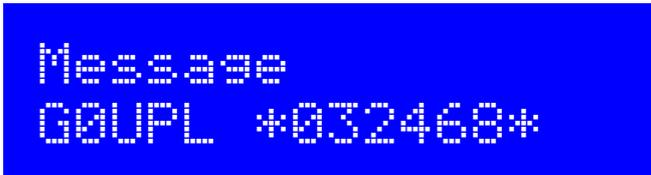
The callsign G0UPL is sent in ordinary FSK/CW with height and speed according to the configuration settings. Next comes a custom message, the duration of each symbol is 03 seconds. The shifts are 1, 2, 3, 4Hz respectively. On Argo, this message produces (with kit configuration FSK (Hz) = 04, Speed = 003):
