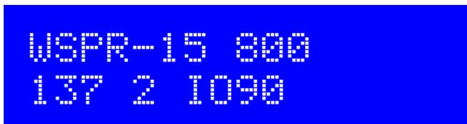
WSPR-15 is a relatively new experimental mode that is a variation of the common WSPR mode. It is used on the LF bands where the higher signal-to-noise ratio it offers is advantageous. WSPR-15 uses the same
