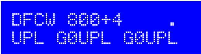
The display will show DFCW followed by the symbol length – in this example 6 seconds. This is followed by the base frequency (see FSK/CW section above) and the FSK size. The scrolling message is shown as usual, with the – or . to show the current symbol of the current character.
