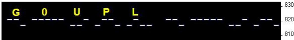
DFCW means dual-frequency CW. The dits and dahs are the same length, but dahs are shifted upwards by the FSK amount. A 1/3 dit-length gap inserted between symbols improves the readability.
