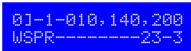
In order to toggle a mode setting between enabled and disabled state: cycle through the menu items with the Left button until you find the mode setting screen you want to enable or disable. Then press the right button twice, to toggle the enable/disabled state.
