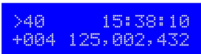
In this example, the calibration just completed has increased the reference clock value by +4Hz to 125,002,432Hz (Ultimate 3 in this example; Ultimate 3S will show a frequency near 27MHz).
