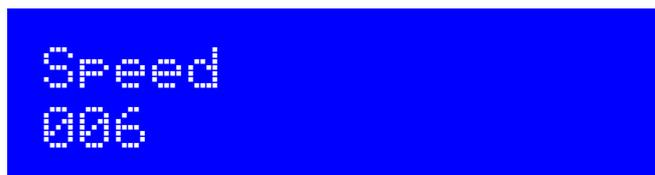
The Speed setting selects the dit speed, in seconds, for the following modes: FSKCW, QRSS, DFCW. In CW and FSK modes, the Speed setting means Words Per Minute. In Slow-Hell mode, the setting is the number of seconds duration of one character (see later section for explanation). The setting has no effect at all, in CW ID, Hell, DX Hell, WSPR, WSPR-15, Opera modes, or PI4 mode; these modes all have a defined timing which cannot be changed. It also has no effect in the TX CW and TX FSK modes.
