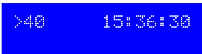
In this example, the time is 15:36:30 and the system is waiting until 40 minutes (time 15:40:00) to start the next message transmission. Additionally the heartbeat will flash, in the space on the top row. When a calibration is about to take place (GPS mode is non-zero) , there will be an additional second line display:
