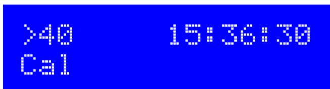
Once the actual frequency calibration starts, the Cal text is followed by a status bar which indicates the progress of the calibration. When calibration has completed, the new reference frequency value for 10 seconds, as well as the change that was made since the previous calibration. For example:
