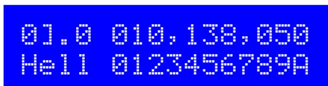
As usual, the display shows the band, mode, frequency and the message scrolls to the left as it is sent.
