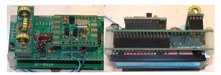
Ensure that the Si5351A synthesiser module is inserted the correct way round as shown in the photograph. The Low Pass Filter kit module should be plugged in with the "Out" legend aligned next to the RF Output connector of the main PCB (see photo).
