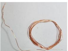
When you have unwound the wire and straightened it, then fold it in half (do not cut it yet). The two halves now need to be tightly twisted together to make the bifilar wire. My method for this is to tie
