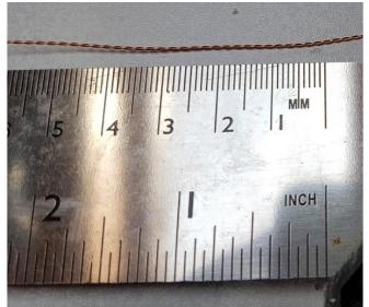
Now cut off the untidy pieces at one and, and the loop from the other: and this is the piece of wire that will be used to wind the FT37-43 toroidal core as a bifilar transformer.
