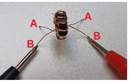
and insert the transformer this way into the PCB. You can carefully cut off those few mm of tinned section of wire, if it won't fit through the PCB holes. But BE CAREFUL not to lose the orientation of the wires! The correct wires must be in the correct holes, so that the windings are connected correctly in the circuit!
