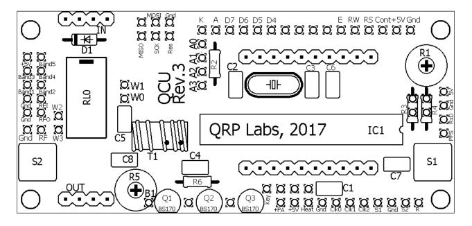
Pay special attention to the orientation of the semiconductors. For IC1, the dimple in the PCB silkscreen must be aligned with the dimple at the top of the IC socket and the IC.
