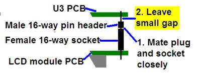
Leave the gap between the male header (plug) and the PCB. I have found this method works successfully.
