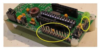
The 16-pin header strip can easily be snapped into smaller pieces. In the photograph (right) I have
