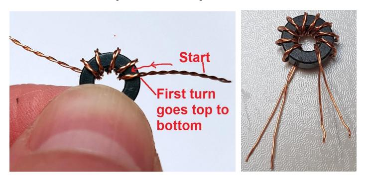
Now it's necessary to identify which wire belongs to which winding. The only way to do this is with a DVM as continuity tester. First, untwist and straighten the wire ends that are not wound around the toroidal core (above right).
