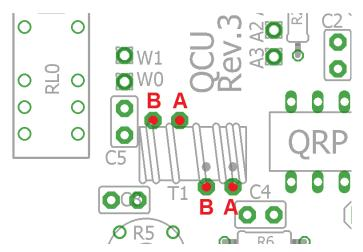
Now trim the wires underneath the board, and tin the ends again. The EASIEST way to do this is simply apply solder so that it sits in the hole and surrounds the 1mm of wire ending, and hold the soldering iron in that position for a few seconds until the enamel is burnt away.
